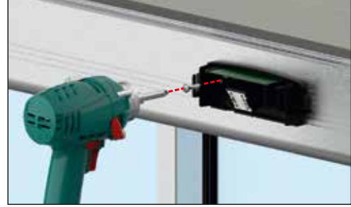
Radar alt kapak alüminyum profile vidalanır. / The motion detector is screwed to the top cover aluminium profile.
